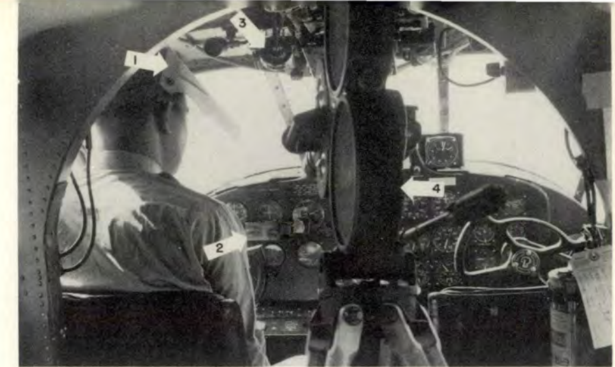
Equipment used to make eye movement studies: 1. Hood, 2. Mirror, 3. Stop Watch, 4. Camera.
