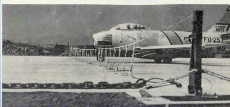
An F-86, moving down the runway at 140 mph, is shown about to make initial contact with nylon webbing of the landing barrier.
