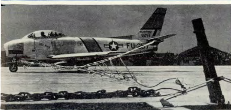
With arresting cable now pulled taut, the F-86 begins to drag the heavy, linked chains stretched along the sides of the runway.
