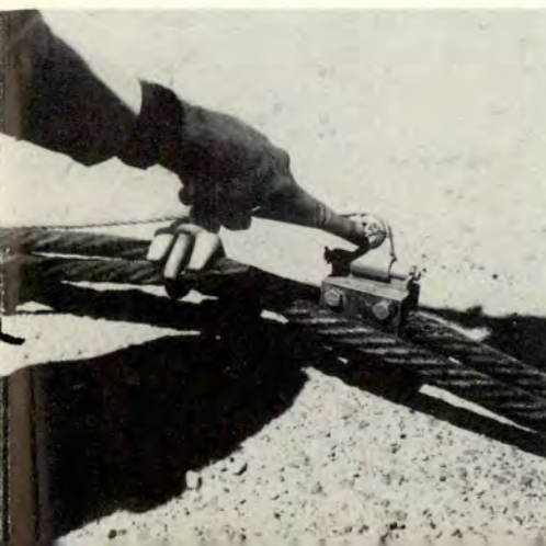
Replaceable shear pin releases actuator strap.
