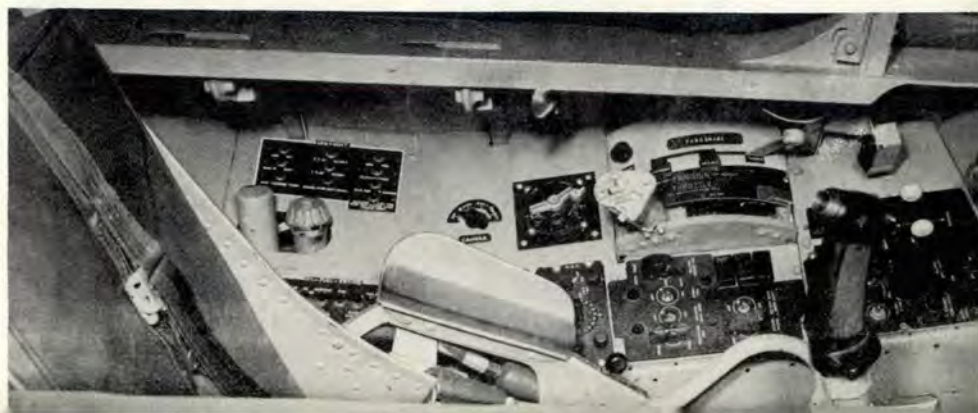
On the page to the left is a photo of the instrument panel of the F-100. Note the simplicity and the standard location of the "basic six." Above and below are right and left consoles.
