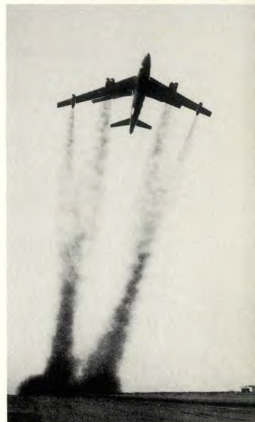
Water injection, 33 ATO units enable B-47E to use shorter fields with maximum loads.
